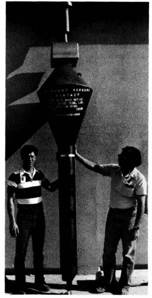
DATABUOY is allowed to free-float on the high seas where it collects nuclear fallout debris data and transmits the information to receiving stations. Two of its developers are Vic Schulze and Harold Gottlieb (both 324).
